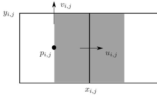
Fig. 1: Notation convection for the pressure, velocity and position of the cell  $(i, j)$ . The shaded region represents the control volume used to discretize the momentum equation in the  $x$ -direction.
