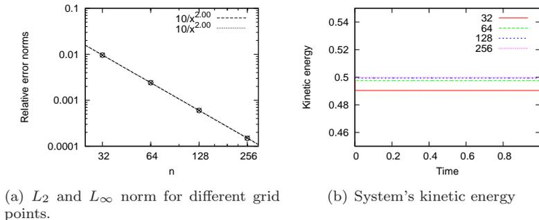
Fig. 2: Green-Taylor vortex. Left: error norms measured at  $t = 1$  for a uniform grid as a function of the number of points per direction  $n$  (symbol  $\times$  is used for the  $L_2$  norm and  $\circ$  is used for the  $L_\infty$  norm). Right: Temporal evolution of the kinetic energy as a function of the level of refinement.
