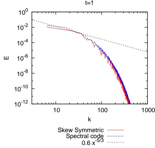
Fig. 8: Energy spectrum obtained from numerical simulation at  $t=1$  with the skew symmetric formulation and a spectral code [5]. Grid:  $256^3$  cells.
