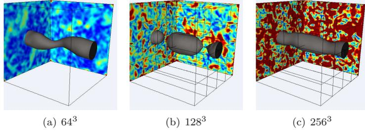
Fig. 13: Snapshots at  $tu'/L_{\text{int}} = 1$  of the interface and vorticity fields in a periodic box for three different levels of refinement.  $r = \rho_l/\rho_g = 10$ ,  $We = 1$  and  $Re_L = 375$ .
