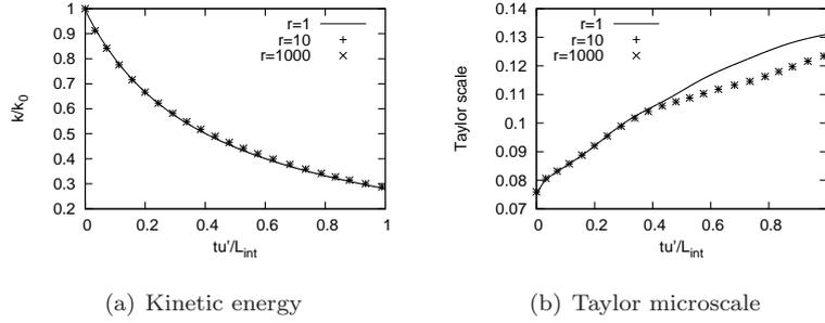
Fig. 11: Temporal evolution of the system kinetic energy and Taylor scale as a function of the density ratio  $r$  for  $Re_L = 375$ .
