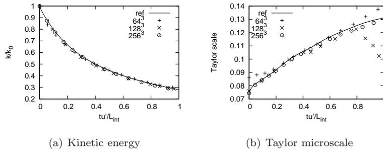
Fig. 14: Temporal evolution of the system kinetic energy and Taylor scale for  $r = \rho_l/\rho_g = 10$ ,  $We = 1$  and  $Re_L = 375$ .
