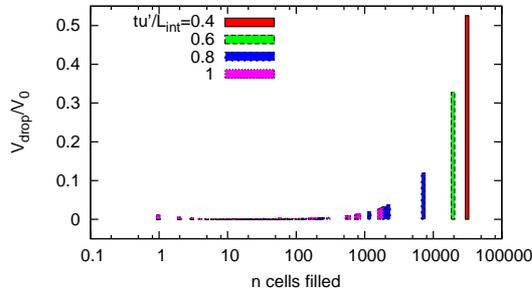
Fig. 12: Histogram of the PDF droplet distribution obtained for  $r = \rho_l/\rho_g = 10$  and  $Re_L = 375$  at different dimensionless times. The x-axis represents the number of *filled* cells used to resolve a given droplet. The y-axis contains the volume ratio between the droplet and the initial rim volume.
