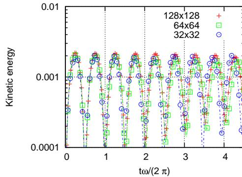
Fig. 4: Oscillation of an inviscid droplet: Temporal evolution of the kinetic energy obtained with the skew-symmetric formulation with  $\beta = 0.15$ . The oscillation period math well with the theoretical frequency.
