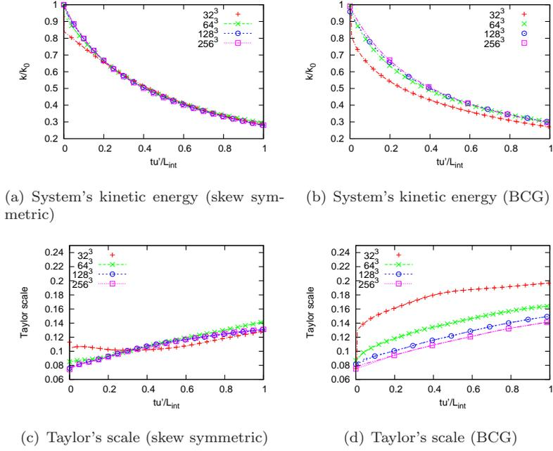
Fig. 7: Temporal evolution of the system's kinetic energy and Taylor's scale as a function of the level of refinement for  $Re_L = 375$  for the skew symmetric formulation (left) and the BCG advection scheme (right).
