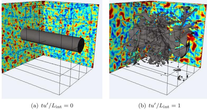
Fig. 10: Snapshots of the interface and vorticity fields in a periodic box for  $r = \rho_l/\rho_g = 10$  and  $\text{Re}_L = 375$ . Grid:  $128^3$  cells.
