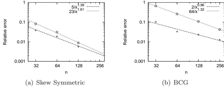
Fig. 9: Relative errors obtained for the kinetic energy (+) and the Taylor scale ( $\odot$ ) as a function of the level of refinement for the skew symmetric formulation (left) and the BCG advection scheme (right).
